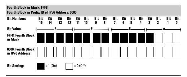
Figure 6-7. Example: How a Mask Determines Authorized IPv6 Manager Addresses by Subnet
